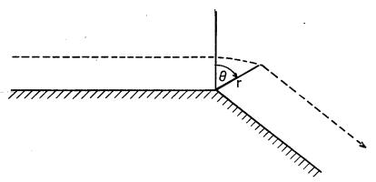
We choose cylindrical coordinates with origin at the corner; u and v are the components of velocity in the r and  $\theta$  directions, respectively, and the equations are
