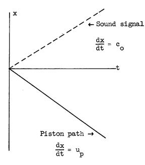
at rest, of a piston being withdrawn from it. Up to t=0, there is a piston at x=0, and gas at rest for x>0. At t=0, the piston commences to move with uniform velocity,  $u_p$ , in the negative x-direction, and a sound signal proceeds into the gas. We now attempt to connect the sound signal and piston-path lines with a family of
