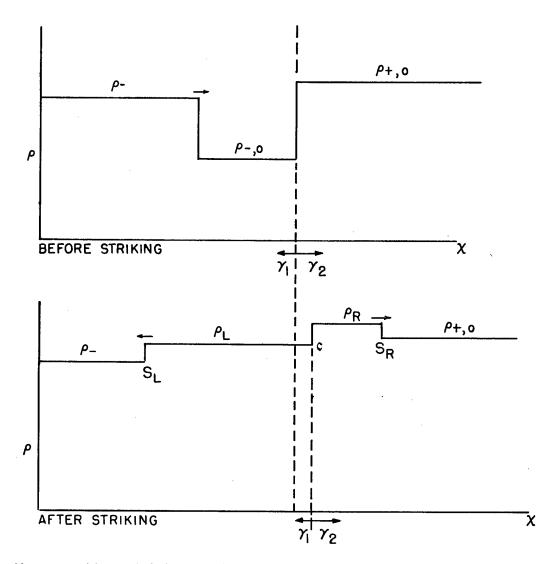
Another question of interest is: How can one use such a reflective system to produce a stationary shock for study? This can be accomplished if the reflected shock at  $s_L$  moves with zero speed. According to (35), the condition for this is  $\rho_u = \rho_L u_c$ . The result of some algebraic manipulation shows that this can be realized provided
