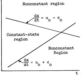
constant-state region with sound speed relative to the material, and thus will have slope u  $\pm c$ , being, therefore, straight characteristics.
