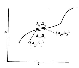
The line in the diagram is a plot of shock position versus time, with the shock moving in the positive x-direction. Draw a rectangle about a segment of the curve in the vicinity of a point of interest.
