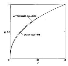
A comparison is shown of the approximate and exact solutions for g(y) for the case  $\gamma = 5/3$ . For smaller values of  $\gamma$ , the agreement is even better, and in the limit  $\gamma \to 1$  the approximate solution becomes exactly correct.
