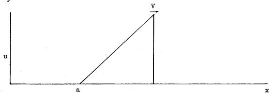
The point at which the velocity drops to zero is x = a. We see from the similarity solution that  $a = \frac{1}{2}$  vt. What is the total displacement of material caused by the passing over of such a detonation wave? This is determined by solving the differential equation:
