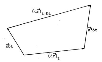
$\overrightarrow{u}$  and  $\overrightarrow{u'}$  are the velocities at each end of  $d\overrightarrow{r}$  at time t. They carry  $d\overrightarrow{r}$  to a new position at time t +  $\delta t$ , such that
