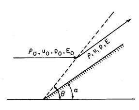
ing gas is moving sufficiently fast, then an attached shock (dotted line) is formed. Since there is no significant length to the system (the appearance of the configuration is independent of magnification), then the shock line must be straight.
